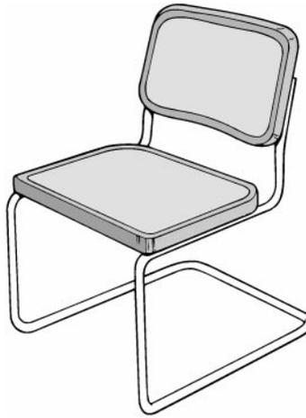
**Fig. 14** The Cesca chair by Breuer, bent metal tubing and rattan, 1924–25.
